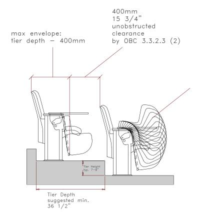
MUST EITHER DROP BY GRAVITY FROM VERTICAL TO STORED or WE MEASURE FROM OPEN POSITION FOR 400MM UNOBSTRUCTED CLEARANCE
